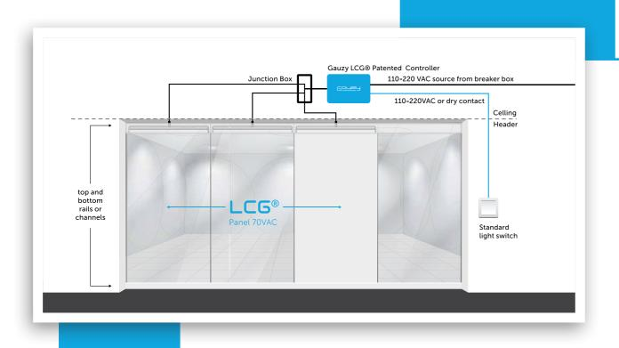
As dynamic as it's users, LCG<sup>®</sup> can be operated with different control interfaces, for spaces that are smart, intuitive, and connected.
